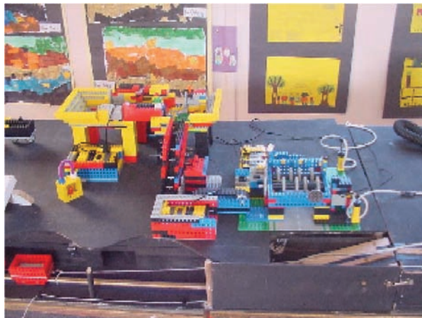
Figure 5: Crusher on the right with a conveyor belt taking the coal over to the main conveyor belt where it is being taken up to the sorting towers. The programmable bricks have been enclosed in a different coloured casing for easy identification by the different groups.
